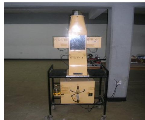
Fig.1: A smoke tunnel
